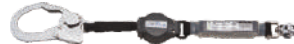
Model No. HL-M RETRACTABLE SINGLE LANYARD - Width 17mm tetoron belt with aramid core length 1,700mm - Equipped with shock absorber - Weight: approx. 920g
