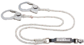
Model No. HL-RW ROPE DOUBLE LANYARD - 10Ø 3 strand nylon rope length 1700mm - Equipped with shock absorber - Weight: approx. 1250g
