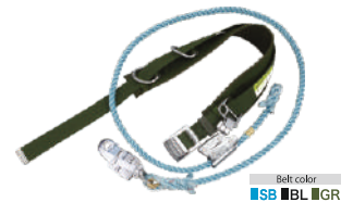
Model No. 4E-GR STANDARD LINEMEN'S SAFETY BELT - Outer Belt: 45mm w x 1300mm L - Inner Belt: 95mm w x 720mm L - Lanyard 16Ø 3 strand nylon rope with red core length 2100mm - Weight: approx. 2,260g
