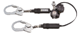
Model No. HL-MW RETRACTABLE DOUBLE LANYARD - Width 17mm tetoron belt with aramid core length 1,560mm - Equipped with shock absorber - Weight: approx. 1,740g
