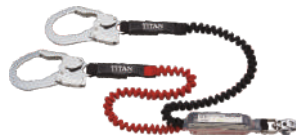
Model No. HL-ERW ELASTIC STRAP DOUBLE LANYARD - Width 27mm polyester coating strap with rubber core - Retracted Length: 1,100mm - Stretched Length: 1,600mm - Equipped with shock absorber - Weight: approx. 1,130g
